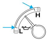
Add oil if needed (refer to *Engine oil* in the *Maintenance and care* chapter). If the oil level is correct, have your vehicle checked at your dealership or by a qualified technician.
